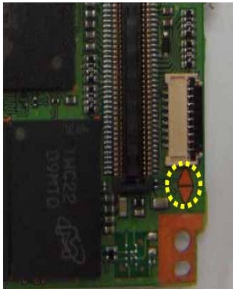
1. Solder the Boot option TP on Main PCB to short out the circuit.
