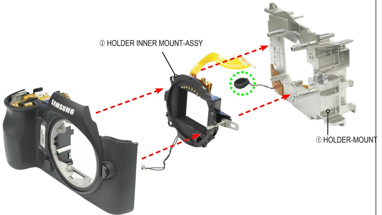
Remove the components in numerical order as it shown in the picture above.
