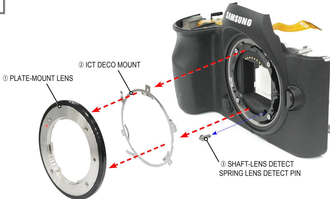
Remove the components in numerical order as it shown in the picture above.
