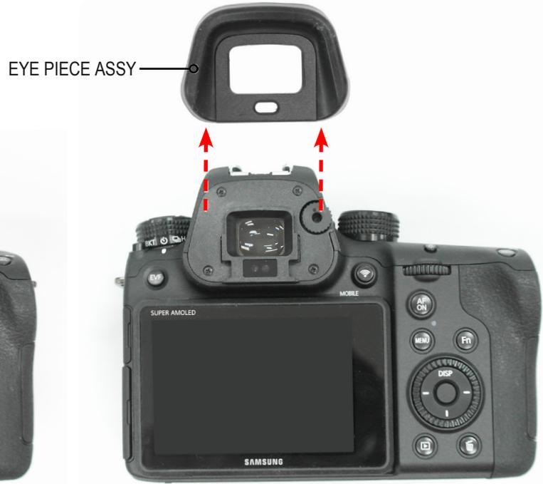
Slide the EYE PIECE ASSY and lift it up in the direction of the arrow as in the picture above.
