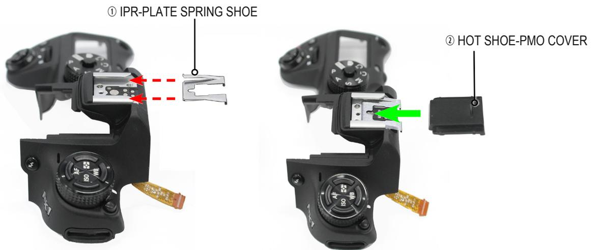
Slide the IPR-PLATE SPRING SHOE in the direction of the arrow as in the picture above. Attach the HOT SHOE-PMO COVER.
