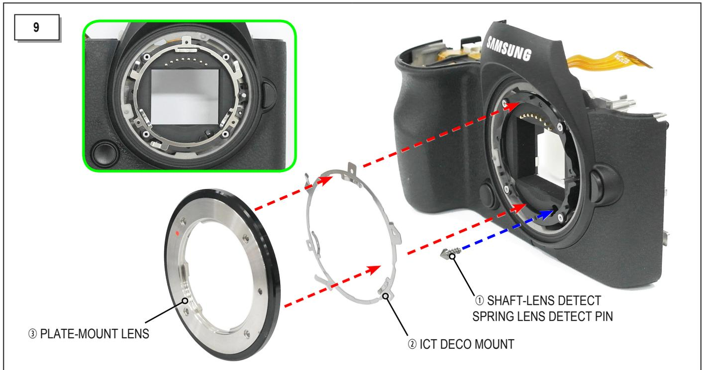
Put the components together in numerical order as it shown in the picture above.
