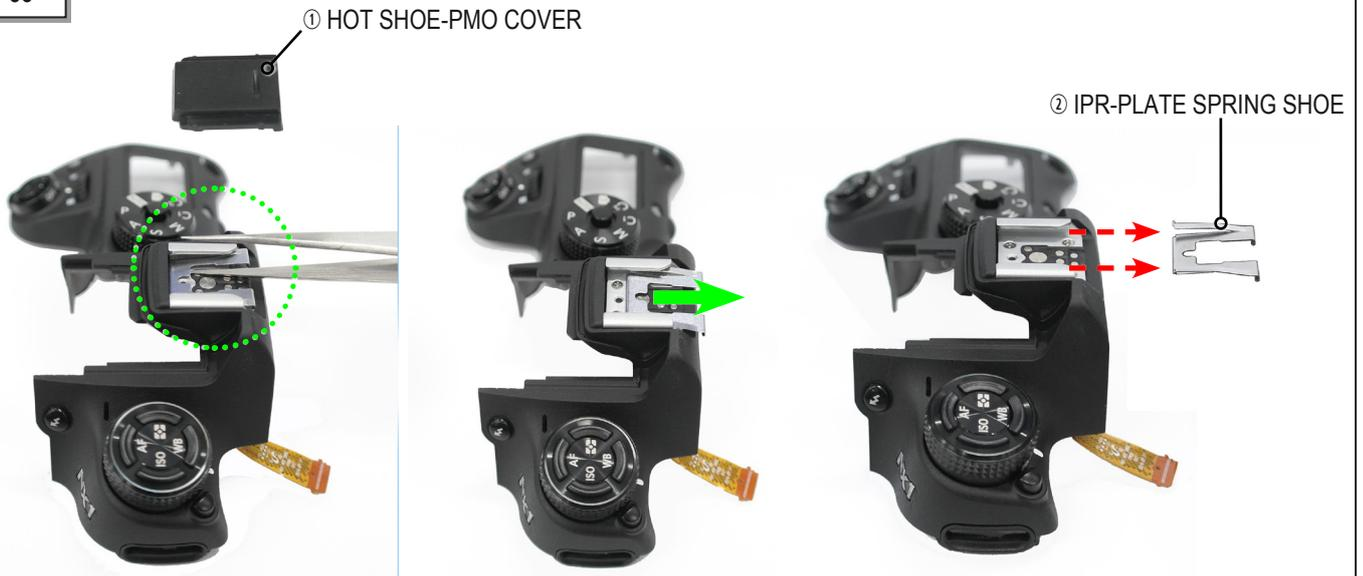
Remove the HOT SHOE-PMO COVER and the IPR-PLATE SPRING SHOE.
