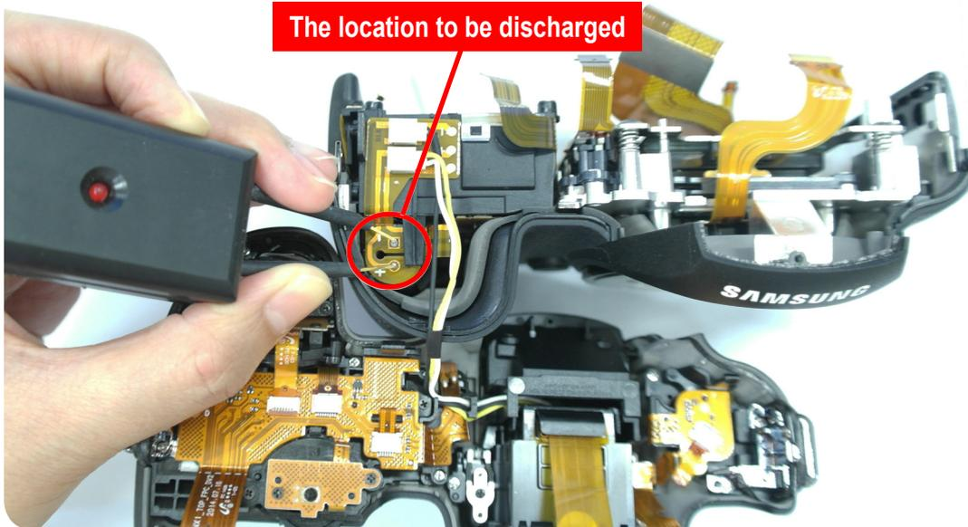
Touch a discharger to the marked area to discharge electricity.
