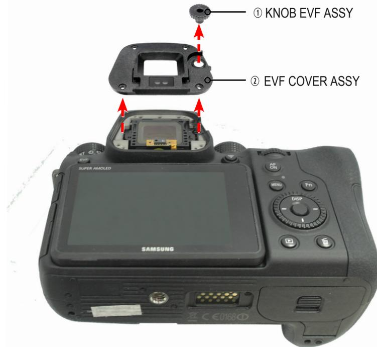
Separate the KNOB EVF ASSY and the EVF COVER ASSY.
