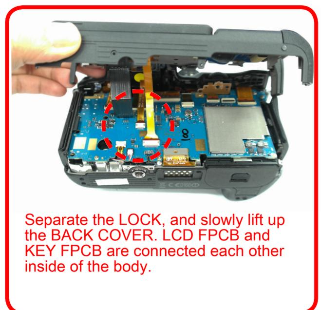
Separate the LOCK, and slowly lift up the BACK COVER. LCD FPCB and KEY FPCB are connected each other inside of the body.
