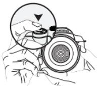
In order to check in advance whether the focus of composition is set appropriately, please use the half-shutter function. If you press the shutter half-way down, the focus and exposure will be adjusted automatically.
