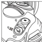
To have a thumbnail view of 9 images, press [□] two times, or press [□] three times to have a thumbnail view of 20 images.
