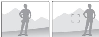
Under the half-shutter state, press the **[AEL]** button of the camera to fix the exposure value and focus information at the same time according to the setting. To cancel the function, press the **[AEL]** button once more. (CD-ROM User manual, page 77)
