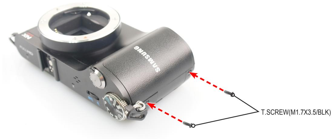
(b) Tighten the 2 screws on the right side and 3 screws on the bottom side of the camera body.
